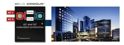
**AC assurance** - HELIX AC utilizes and monitors two ac branch circuits. Trouble to a primary branch instantly switches power to the back up branch to maintain uninterrupted AC operation.
