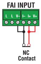
FAI Activates when the NO contact CLOSES. FAI Deactivates when the NO contact OPENS AND the NC contact momentarily OPENS.
