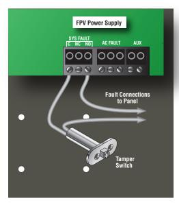
Figure 1 - Tamper switch fault relay wiring
