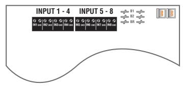
Each input on the **R8 / R8P** has an "**IN**" terminal and a "**GND**" terminal.
