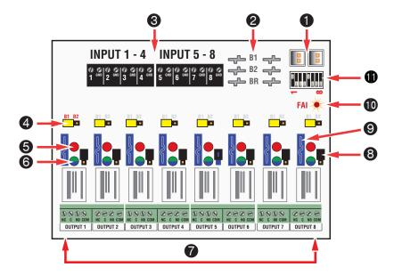
The relay contact outputs have suppression diodes across them. For a dry contact output, the output diodes must be cut and the yellow and black jumpers removed.
