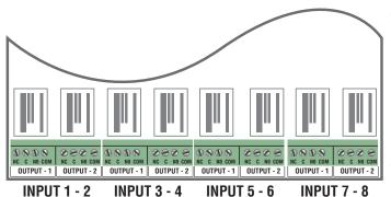
Each output on the **R8 / R8P** has "**NC**", "**C**", "**NO**", and "**COM**" terminals.
