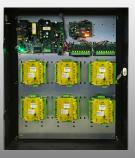
Seamless design - mechanical integration of power, locks and Paxton controllers into one innovative unified system.
