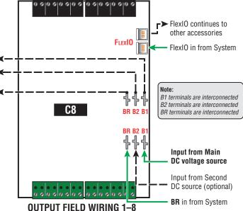
Each of the B1, B2, BR, and FlexIO busses has two connectors. These connectors may be used interchangeably.
