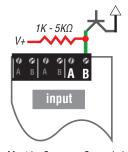
Must be Common Grounded with FPO Power Supply
