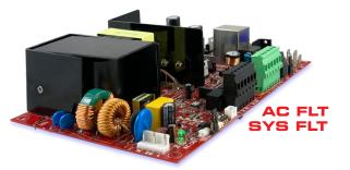
Every **FLEX**POWER power supply has two Form C relay contacts to annunciate System Fault and AC Fault. These fault contacts may either be monitored separately or wired together for common fault monitoring.
