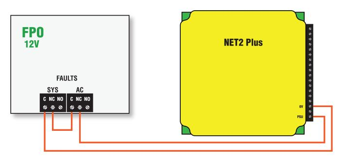
Note: FPO Fault relays are labeled in the unpowered (fault) condition
