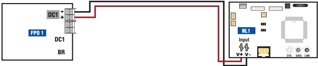
Figure 1.5 - Power the NL1 off the FPO DC1 terminals
