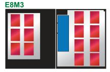
**NOTE** - Although the E8M3 will physically hold up to 14 Mercury controllers, there may not be enough power or distribution space available for all configurations.
