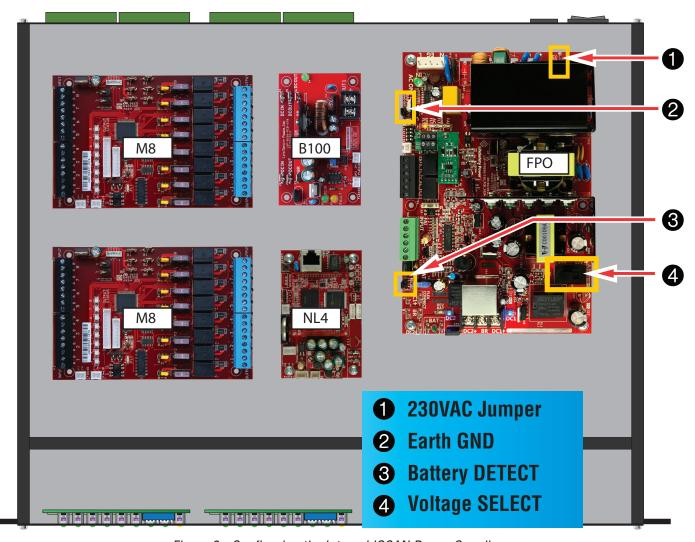
Figure 3 - Configuring the Internal ISCAN Power Supplies
