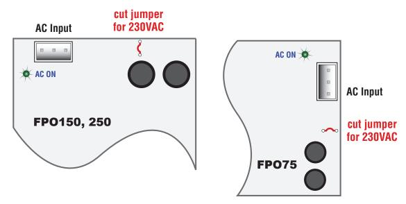
Figure 4 - FPO 230VAC jumper location
