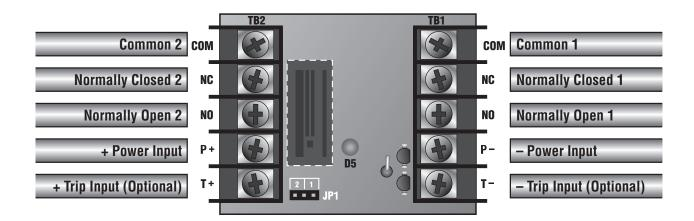
Wiring to the Power and Trip Inputs shall be contained within the same room, max. wiring distance of 3 meters. Class 2 power limited wiring must be separated from non-power limited wiring by a minimum of 1/4 in and must use separate knockouts. Refer to power supply installation instructions for further guidance.
